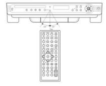
The batteries normally last for about six months. This depends on how often and for what operations the remote control is used.
